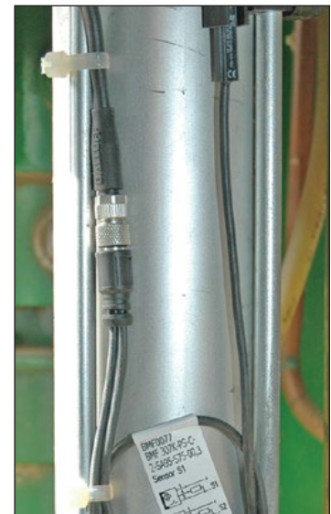
A better solution is to use cylinder mounted magnetic field sensors that can replace two proximity switches, targets, or additional mounting hardware
