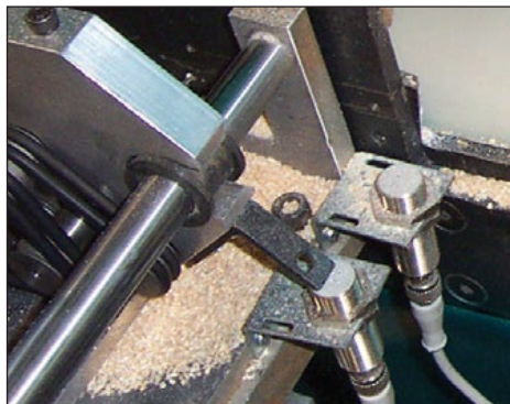
Traditionally, two proximity switches detect flags for end of stroke of a pneumatic carriage
