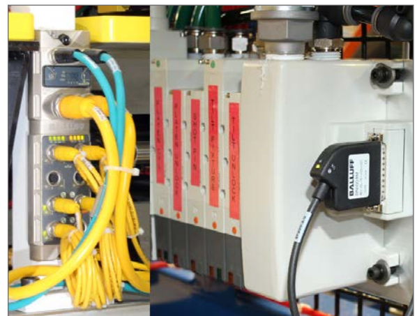
Figure 3: Valve Control with Distributed Modular I/O saved the customer over $350 per manifold.
